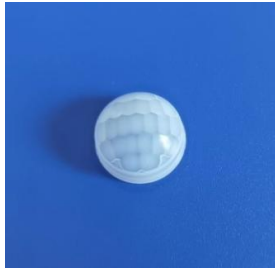
Model No.:YY-2100 Size: \text{Ø}21*11.8 Focal length: 11mm Angel : 120^\circ Distance: 10.8m
