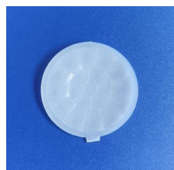
Model No.:YY-1204 Size: Ø33.6 Focal length: 18mm Angel: 360° Distance: 14m ceiling mountng 10m
