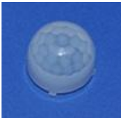
Model No.: 8003-1 Size: \varnothing 22.7*18.6 Focal length: 10.5mm Angel: 100° Distance: 10m
