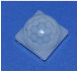
Model No.: 8002-2 Size: 23.3*23.3*14.8 Focal length: 10.5mm Angel: 110 ° Distance: 11m
