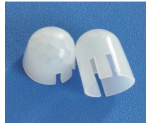
Model No.: 8308-2 Size: ∅11.5*14.5 Focal length: 6mm Angel: 60 ° Distance: 5m
