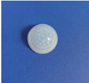
Model No.: YY-B2010 Size: Ø23.4*13 Focal length: 10mm Angel: 360° Distance: r:5m
