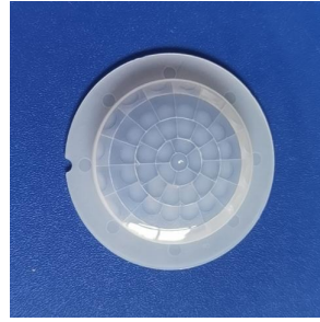
Model No.:YY-D36 Size: Ø36*7.2 Focal length: 17.5mm Angel: 360° Distance: 10m
