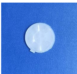
Model No.:YY-1201 Size: Ø17 Focal length: 8mm Angel: 360° Distance: 7m ceiling mounting 4m
