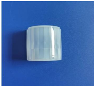
Model No.: LC-2818 Size: 31.3*27.7*19.9 Focal length: 13mm Angel: 120° Distance: 10m
