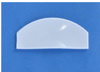
Model No.:SIR650 Size : 46*20 Focal length:30mm Angle:15 ° Distance:12m
