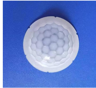
Model No.:8603-6G Size: Ø38.8 Focal length: 17.5mm Angel: 360° Distance: 14m
