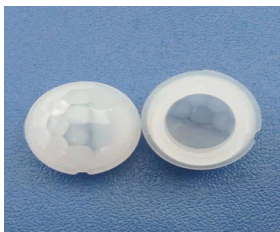
Model No.: 13120F-3 Size: 14*10.4 Focal length: 6mm Angel: 120° Distance: 8m
