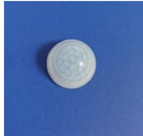
Model No.: YY-B2010 Size: \varnothing 23.4 \times 13 Focal length: 10mm Angel : 120° Distance: 10m
