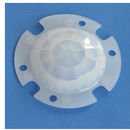
Model No.: 8603-3 Size: \varnothing 45.9*11.4 Focal length: 17.5mm Angel: 360° Distance: Dia10m
