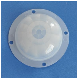
Model No.: 8605-3W Size: \varnothing 43.6*11.4 Focal length: 15mm ceiling mounting 2.5M Angel: 360 ° Dia: 10m
