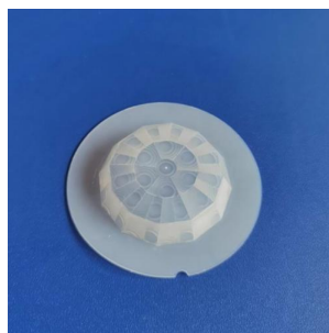
Model No.:7906-20-G3 Size: Ø52.5 Focal length: 19.6mm Angel: 360° Distance: radius 5.9m
