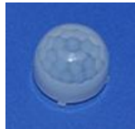
Model No.: 8003-1 Size: \varnothing 22.7*18.6 Foca length: 10.5mm Angel: 100° Distance: 10m
