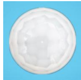
Model No.: 01809-2 Size: 17.8*11.95 Focal length: 9mm Angel: 120° Distance: 8m
