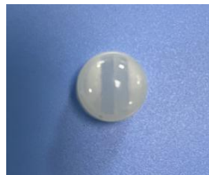
Model No.: 8121-5 Size: 9.8 Focal length: 5.2mm Angel: 120° Distance: 8m
