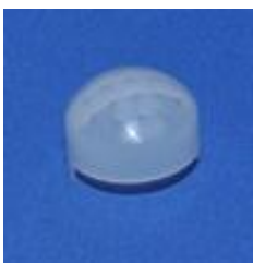
Model No.: 7709-1 Size: \varnothing 20.7*16.9 Focal length: 7.6mm Angel: 120 ° Distance: 8m
