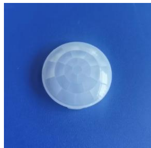
Model No.:LTX-01 Size : Ø33.05*9.75 Focal length:12.7mm Angle:120 ° Distance:5m
