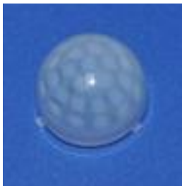
Model No.: 9002-1.7 Size: \varnothing 24*20 Focal length: 12mm Angel: 360° Distance: 10m
