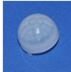
Model No.: NL-02 Size: 23.3*19 Focal length: 11.6mm Angel: 120° Distance: 10m
