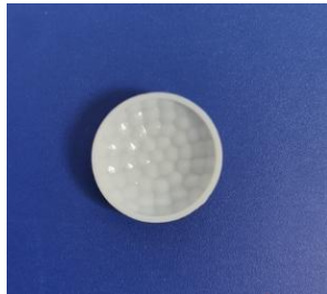
Model No.: 29207 Size: Ø29.4*7.53 Focal length: 8mm Angel: 120° Distance: 8m
