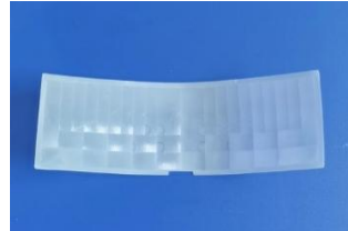
Model No.:AF-2430 Size:116.5*38 Focal length:30mm Angle:180 ° Distance:20m 2 pieces of PIR
