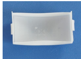
Model No.: AL23 Size: 34.5*20*10.5 Focal length: 20mm Angel:horizontal120° Distance: 7-10m
