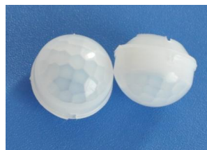
Model No.: 018090 Size: \varnothing 17.8*13.94 Focal length: 9mm wall/ceiling mounting 3m Angel: 360 ° Distance: 8m/Dia6m
