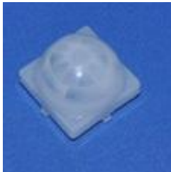
Model No.: 023100 Size: 23.4*23.4*18.9 Focal length: 10.5mm Angel: 120 ° Distance: 10m
